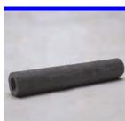
Fibre cement tube for reinforcement of waterproof walls. Acts as formwork spacer and as cover for the tie rod. In this way the thickness of the concrete walls and the reuse of the tie rods in guaranteed.
